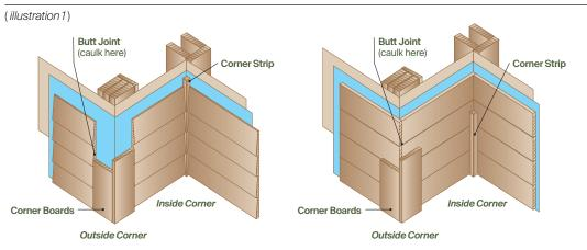
Inside corner treatments are generally easier. Siding is typically butted against a 2x2 inch trim strip, or it can be butted directly against the adjoining wall with a trim strip covering the joint.
